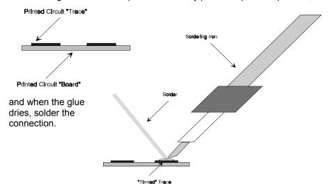
This may go a little "against the grain" at first, but it is by far the easiest method. Notice also that when reheating the solder that the iron tip does not come in contact with the "tab" on the body of the chip component. Over heating of this solder tab can cause a fracture of the bond to the component, causing an intermittent connection.
